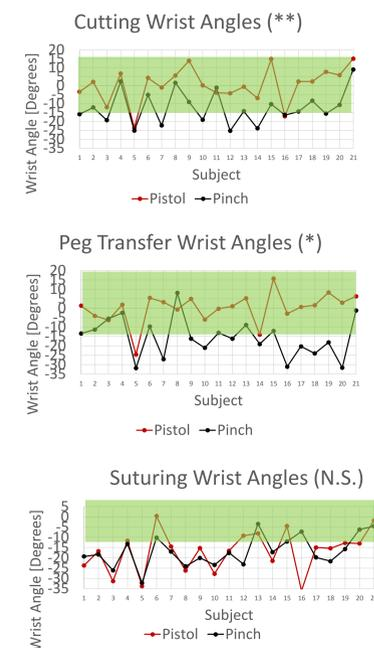
Figure 5. Within subject comparison of wrist flexion/extension angles experienced when using each tool, the green area represents neutral wrist posture ( $-15^\circ < x < +15^\circ$ ); \* denotes significance ( $p < 0.05$ ) and \*\* ( $p < 0.01$ )
